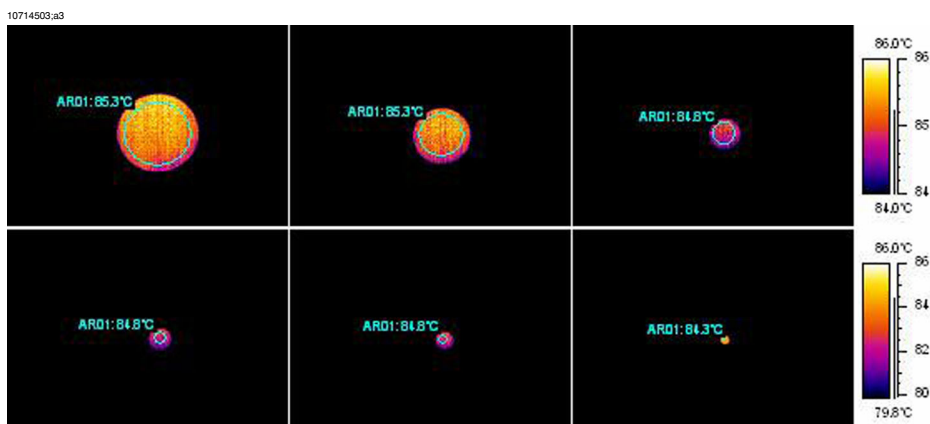
Figure 7.19 Temperature readings from a blackbody at +85^{\circ}\text{C} ( +185^{\circ}\text{F} ) at increasing distances
